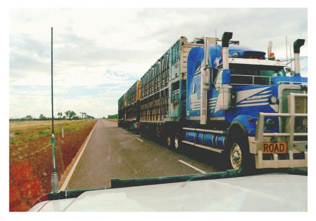
Passing a road train on an SA outback highway, 70+ tonnes, 62 wheels, travelling at 90km/h. Good thing both drivers were well trained by road safety professionals. Image: Hughes Training Group
